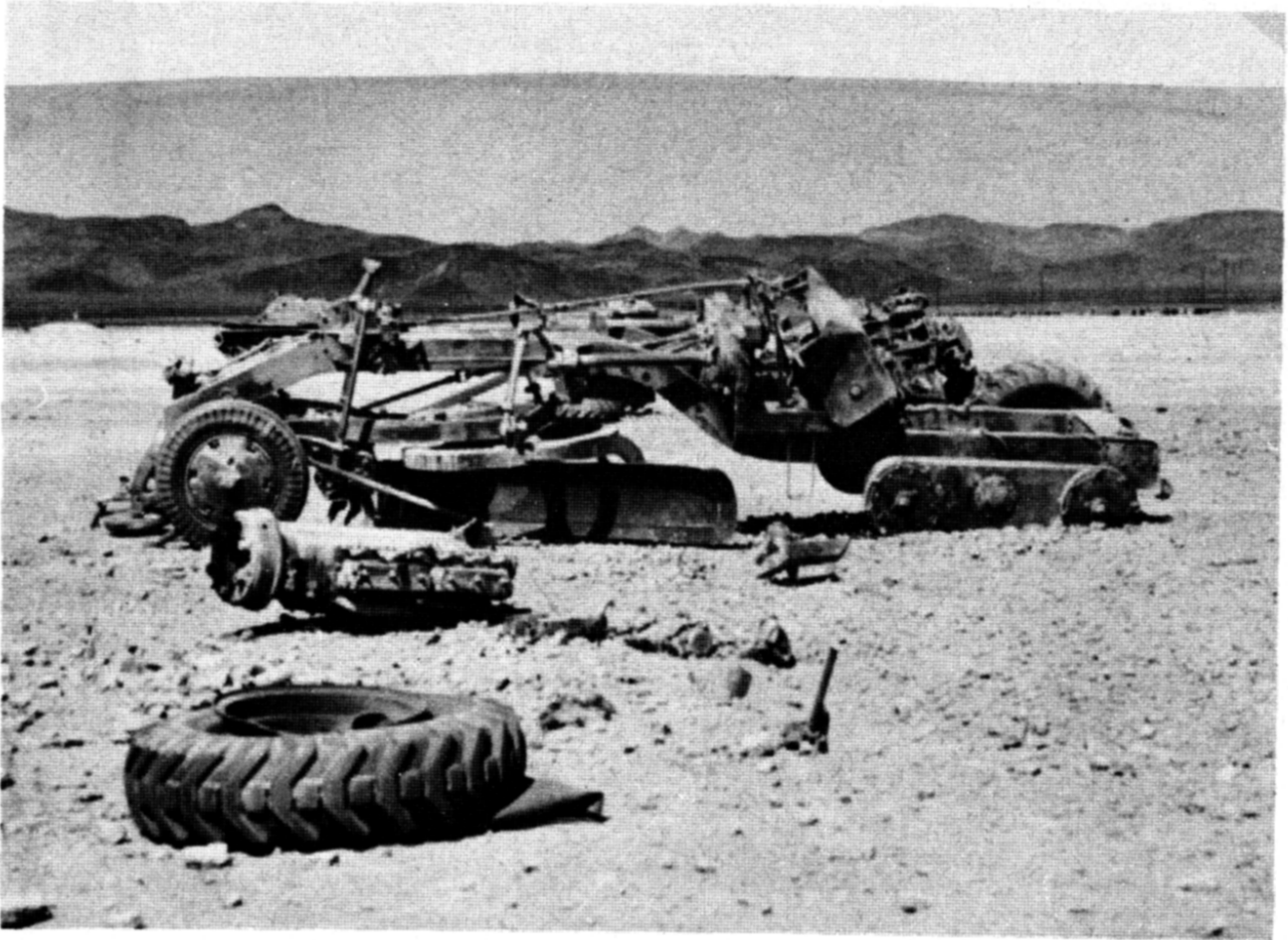
Figure 12.40a. Earth-moving equipment subjected to nuclear blast in open terrain (30 psi overpressure).
